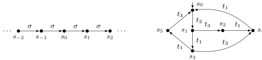
Fig. 2. On the left, a two-way uniform chain based on \sigma . On the right, a labelled transition system with states \{s_0, s_1, s_2, s_3, s_4, s_5\} , labels \{t_1, t_2, t_3\} and initial state \iota = s_0 . It is isomorphic to the reachability graph of Figure 1. The label t_2 is enabled at s_0 and t_3 is backward enabled at s_0 . The state s_1 is reachable from s_0 through the execution of t_2 . Denote by \sigma the sequence t_2t_3t_1t_1 . Then, the Parikh vector of \sigma is \mathbf{P}(\sigma) = (2, 1, 1) and its support is \text{supp}(\sigma) = \{t_1, t_2, t_3\} . Since s_0[\sigma]s_0 , \sigma is a cycle around state s_0 . This lts is totally reachable, weakly periodic, fully deterministic and fully backward deterministic, strongly cycle consistent, persistent, backward persistent and reversible.
